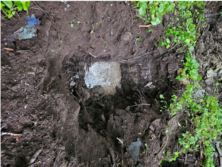
Photo 5: Test Pit TP-15 containing fill material including black asphalt roofing material, sheet metal, plastics, glass bottles, brick.
