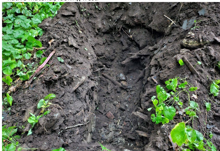
Photo 4: Test Pit TP-13 containing fill material including black asphalt roofing material, brown rubber material, sheet metal, plastics, glass bottles, brick.
