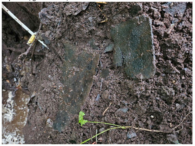
Photo 6: Black asphalt roofing material from Test Pit TP-13.
